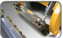
POWER-A-TACH® SYSTEM Power-A-Tach® system option allows users to quickly install and remove attachments. An operator leaves the seat only to connect auxiliary hydraulics.
