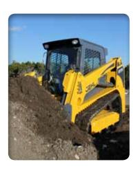
antistall technology senses machine load electronically, monitoring and adjusting the hydrostatic drive pump resulting in tractive effort of 11,840 lbs. (5371 kg) on the RT175 and 12,359 lbs. (5606 kg) on the RT210.
