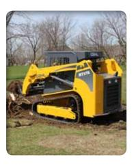
TRACK LOADER CHASSIS aids in superior weight distribution which enhances stability, grading, tractive effort, and ride control.
